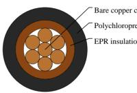
Bare copper conductor Polychloroprene rubber outer jacket EPR insulation
